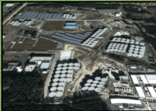
Storage tanks holding radioactive water at Fukushima Daichi nuclear plant. Typhoons and heavy rainfall have caused the tanks to leak, releasing high levels of strontium and tritium into the environment. Photo credit: Wikimedia Commons.
